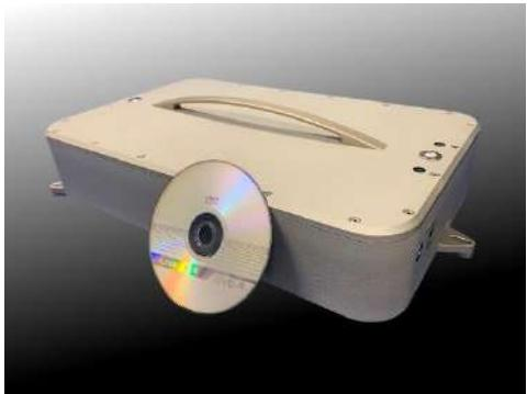
The all-new Tenacity uses Ti:Sa direct diode pumping technology and delivers remarkable performance from a surprisingly compact package. The monolithic design of this femtosecond oscillator gives it unrivaled stability and it also benefits from active output power control to further improve long-term stability. It is now available in several versions delivering up to 500 mWatts at 800 nm / 80 MHz with a 50 nm spectrum allowing compression down to < 15 fs.
